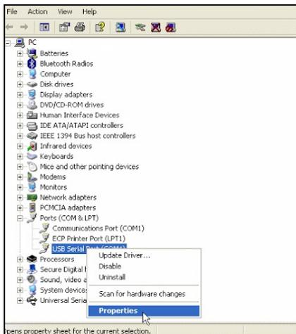
Fig. 10a - Accessing Advanced COM port setting
