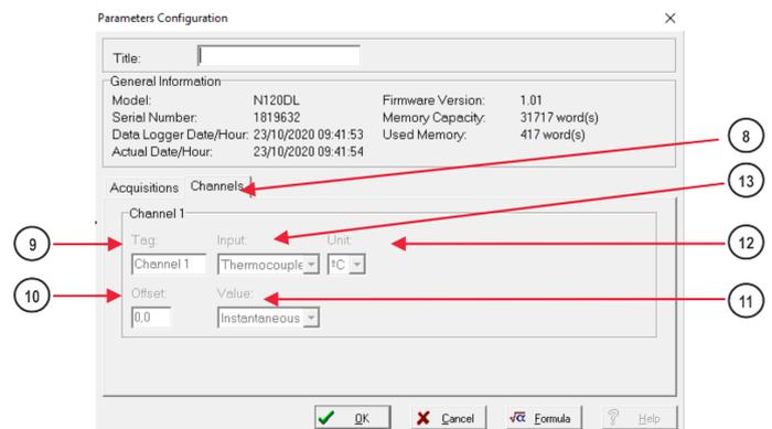
Fig. 5 – Controller Configuration (Channels)
