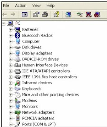
Fig. 9b - Determining the COM port
