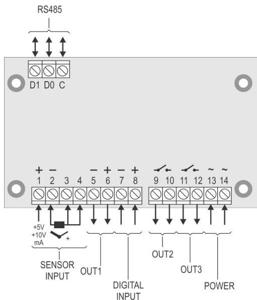
Fig. 3a – Input, outputs, power supply and RS485 interface
