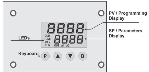
Fig. 1 – Front panel elements
