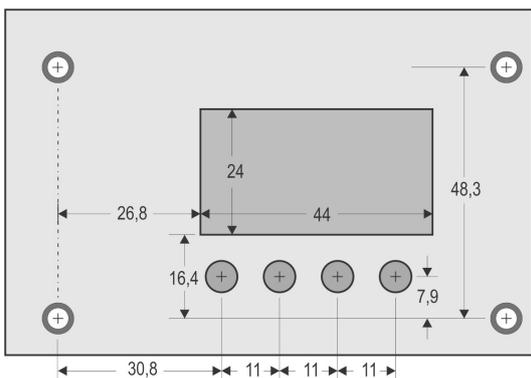
Fig. 2b – Keypad, display and LED distances (Frontal view)
