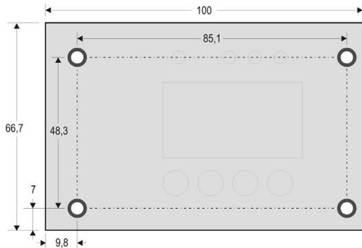
Fig. 2a – Screws mounting holes (Frontal view)
