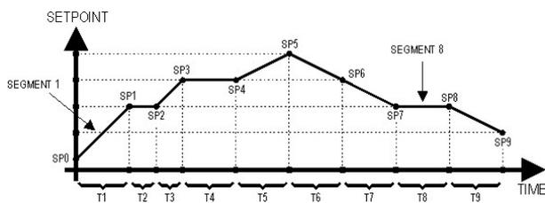
Fig. 4 - Example of a Ramp and Soak program
