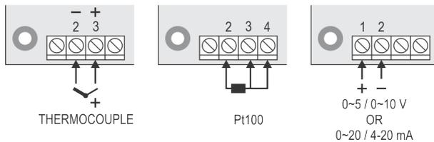
Fig. 3b – Input, outputs, power supply and RS485 interface
